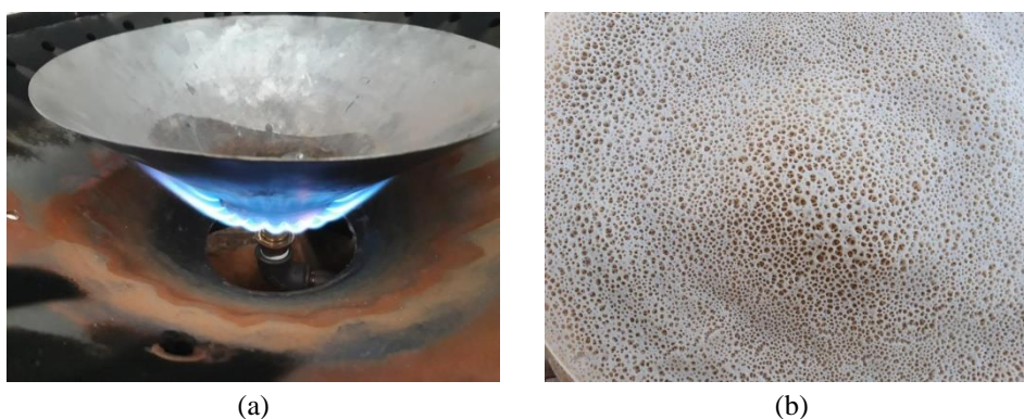
Fig. 6 Burning flame with fixed cone (a) and injera baked using adjustable cone (b)
