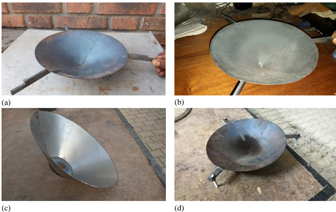
Fig. 3 different arrangement of inner cones (a) small cone (b) big cone (c) fixed cone (d) adjustable height
