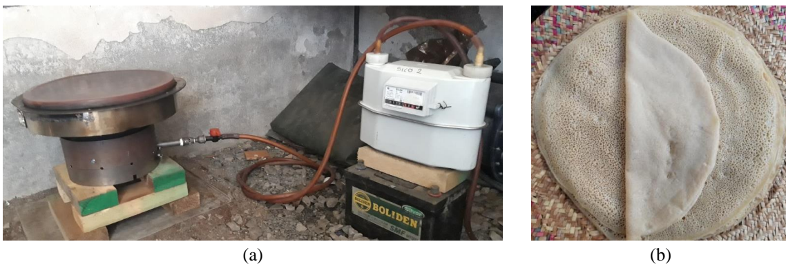
Fig. 5 Injera baking mitad connected with biogas flowmeter (a) and Injera baked with lower cone (b)
